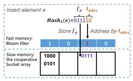
Fig. 1: Insertion of the Elastic Bloom filter. The Bloom filter size m=4, the length of hash functions w=6 and number of hash functions k=1. When inserting an item e, we first calculate its binary hash number  $011110_2$  by  $h_1$ . Next, we divide the hash number by m to get the  $F_p=0111_2$  and  $I_{ndex}=10_2$ . Then, we set  $A[10_2]$  to 1 in the Bloom filter and insert the fingerprint  $0111_2$  into bucket  $B[10_2]$ .
