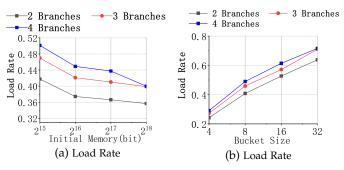
Fig. 9: Load rate comparisons for different numbers of branches in the bucket tree. We vary the Bloom filter size and the bucket size to figure out the relationship between these variables.
